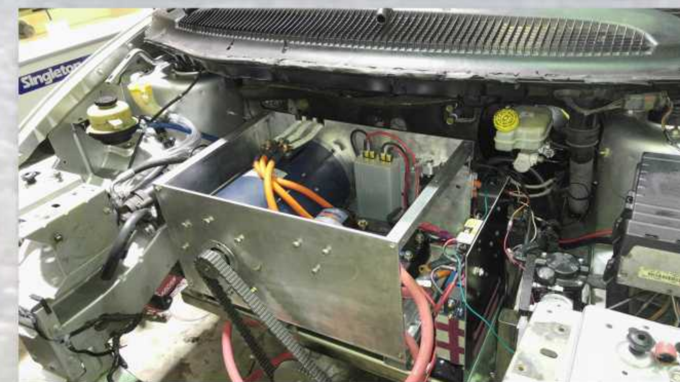
Figure 3: SolidWorks render vs. manufactured battery housing (left) and "powertrain box" (right)
