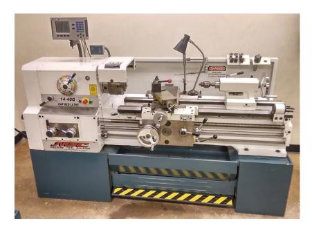
Normally, a part is held in a collet or lathe chuck and a cutting tool is held in a tool post. The lathe is switched on and the part begins to rotate. The cutting tool is then brought to the rotating part and removes material.
