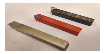
**THE LATHE BIT** The image above shows the most common lathe cutting tools, they are called lathe bits.
